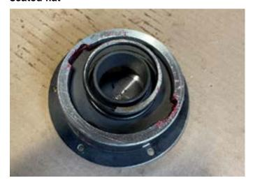
17. Apply 1 drop of Loctite 242 or equivalent onto the threads of the lockout bolts. Carefully install the assembly onto the hub, ensuring that the thick engagement spring is centered against the coupler gear inside the hub.
