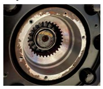
11. Install the externally splined coupler gear into the hub. Note that the spring will slightly push the coupler back out after letting go, but it will stay in place.
