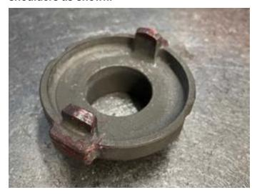
13. Grease the bezel slots and selector ramps as shown
