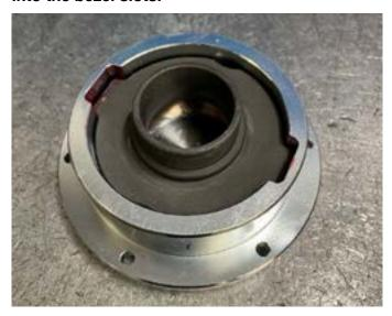
15. Install the bezel to hub gasket, using the mounting bolts to align and hold the gasket in place during assembly.
