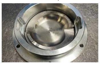
7. Install the selector retaining ring by first feeding one end into the groove within the bezel bore. Then, press the exposed end down until the ring snaps into place. Rotate the ring so the ends are 90 degrees from the vertical grooves in the bezel.
